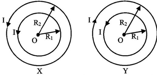
Consider the two different situations X and Y of two concentric coils of  $N_1$  and  $N_2$  turns and radii  $R_1$  and  $R_2$  respectively as shown above. If the magnetic field at O in situation X is  $B_x$  and in situation Y is  $B_y$  then  $B_x - B_y$  is
